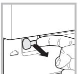
4. pull outwards using the tab as indicated in the figure, until the plastic tie-rod is freed from its stop position; pull downwards until you hear a "click", which indicates that the door is now unlocked.
